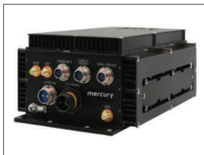
▲ Fig. 3 A ruggedized RFSoc enclosure for mounting directly behind a phased array EW antenna delivers digitized signals across dual 100 GbE optical interfaces using the VITA-49 data protocol.
