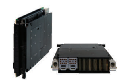
▲ Fig. 4 An RFSoc SOSA aligned 3U OpenVPX plug-in card has 20 VITA 67.3 backplane RF coaxial connectors and two 100 GbE optical I/O ferrules.
